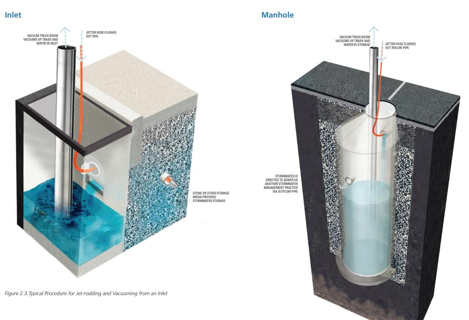
Figure 2.4. Typical Procedure for Jet-rodding and Vacuuming from a Manhole
