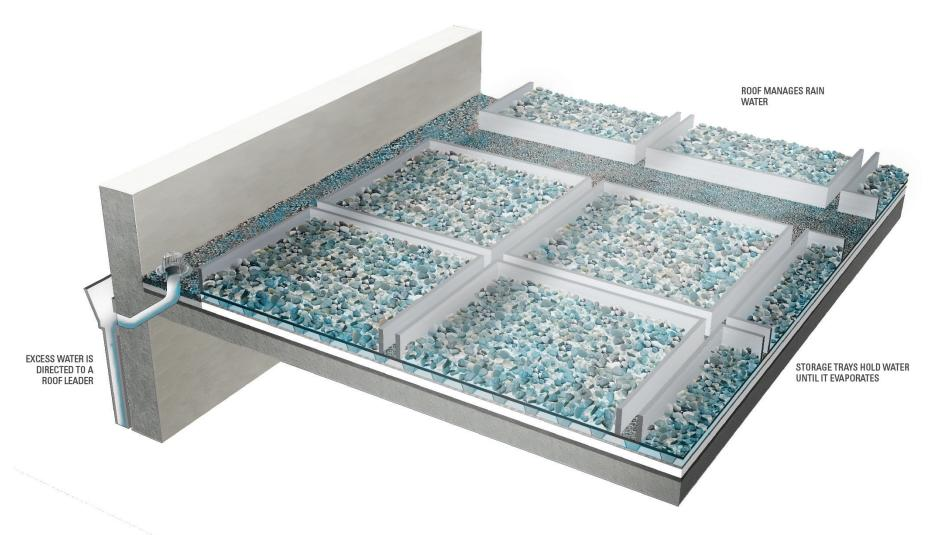
Figure 1-27. Blue Roof Detention Tray, Check Dam, and Modified Roof Leader System Sections/Perspectives with Typical Features
