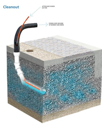
*Figure 2.5. Typical Procedure for Vacuuming and Jet-rodding form a Cleanout Access Structure*
