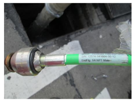
Figure 3-7: Small rotating, root cutting nozzle
