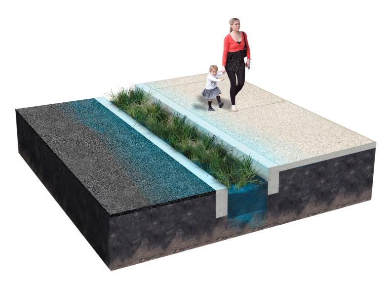
Figure 1-29. Green Gutter Section/Perspective with Typical Features
