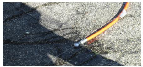
Figure 3-3. Small penetrating nozzle with one front facing and six rear- facing jet-rods
