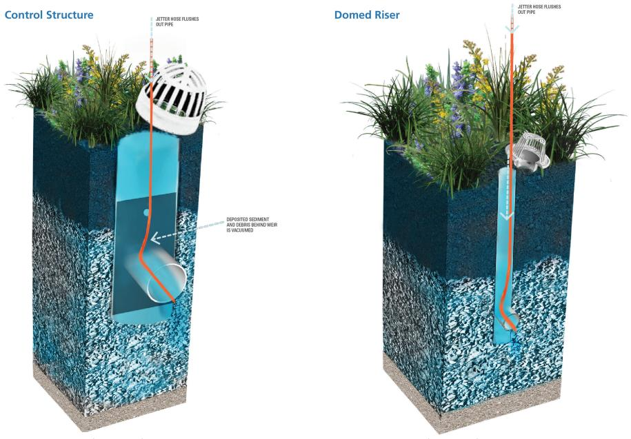
Figure 2.1. Typical Procedure for Jet-rodding from a Control Structure with a Weir
