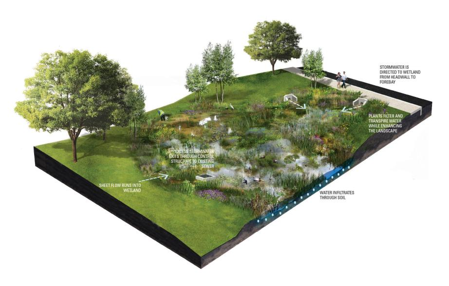
Figure 1-13. Stormwater Wetland with Typical Features
