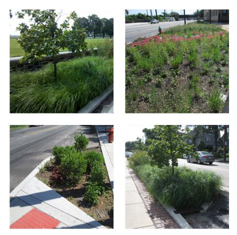
Figure 1-7. Examples of Stormwater Bump-outs in Philadelphia
