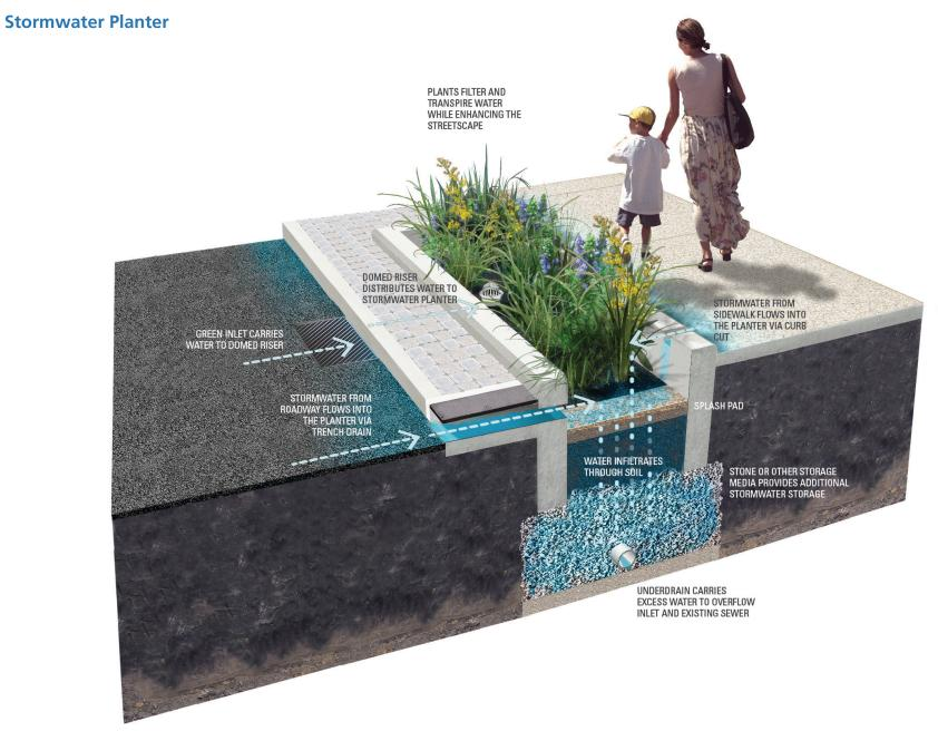
Figure 1-6. Stormwater Planter Section Typical Features
