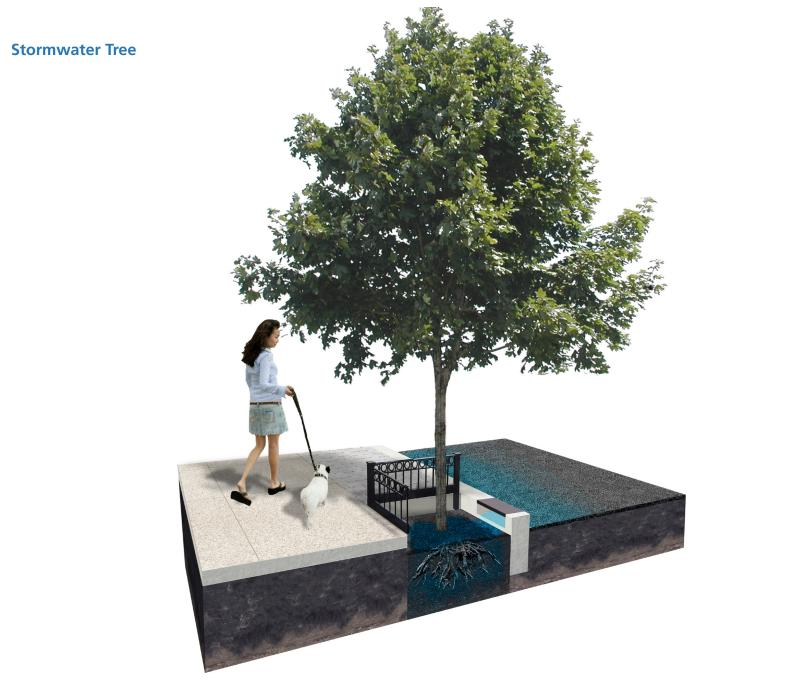
Figure 1-19. Stormwater Tree with Typical Features
