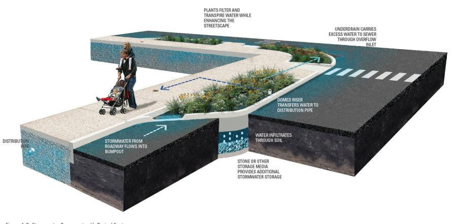
Figure 1-9. Stormwater Bump-out with Typical Features
