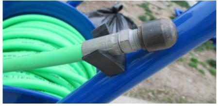
Figure 3-1. Small flushing nozzle
