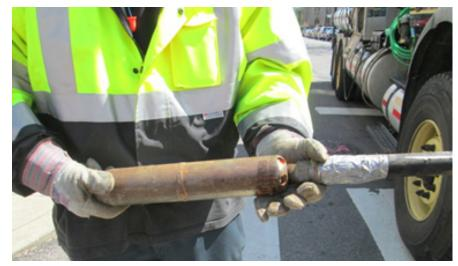
Figure 3-4. Large penetrating nozzle with one front-facing and five-rear facing jet-rods
