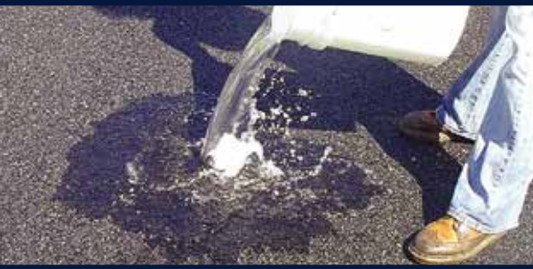
Examples of porous pavement
