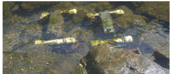
Figure 2. Weighted PVC pipes help keep the biofilm samplers in place.
