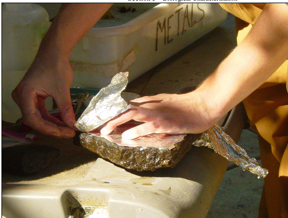
Figure 5.38 Cutting Foil to Algal Periphyton Sampling Surface Area
