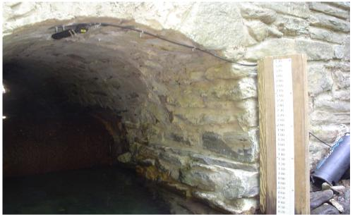
Appendix A, Figure 10 - An ultrasonic down-looking acoustic water level sensor for water level measurement as it was installed above the Cathedral Run tributary
