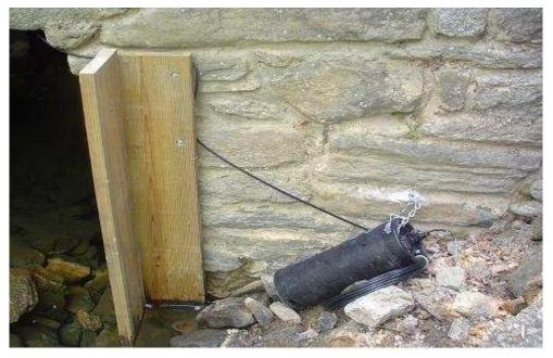
Appendix A, Figure 11 - A pressure transducer for redundant water level measurement as it was installed in the Cathedral Run tributary.
