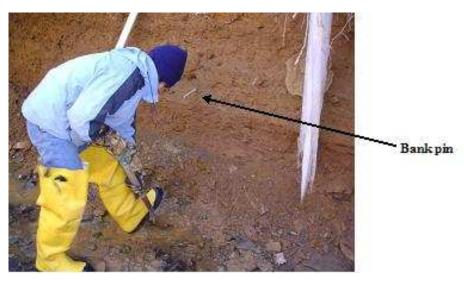
Appendix A, Figure 1 - PWD staff digging out eroded bank sediment in order to accurately measure bank pin exposure
