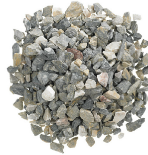
ASTM NO. 8 STONE 3/8 - 1/2 INCH AVERAGE
