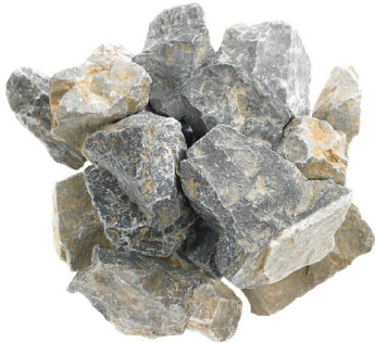
ASTM NO. 2 STONE 2 - 3 INCH AVERAGE
