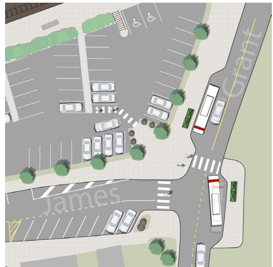
Excess asphalt is to be used to improve pedestrian safety and urbanize the intersection at James and Grant.
