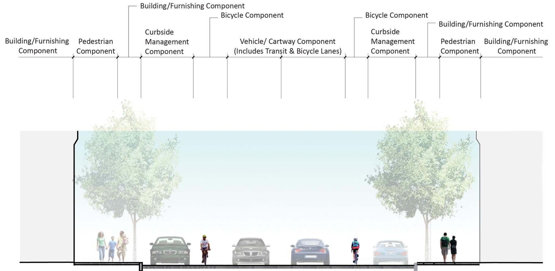
Figure 4.2: Plan View of typical SMP layout within street right-of-way
