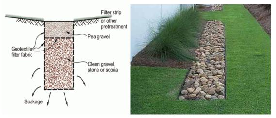
**Infiltration Trench**: A subsurface structure designed to detain runoff and allow infiltration, if possible. The outflow component controls stormwater runoff peak rates and quantity.
