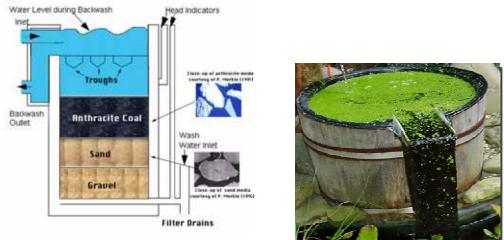
**Sand Filters**: Sand filters work by providing the particulate solids with many opportunities to be captured on the surface of a sand grain. As fluid flows through the porous sand along a tortuous route, the particulates come close to sand grains. Then they can be captured.
