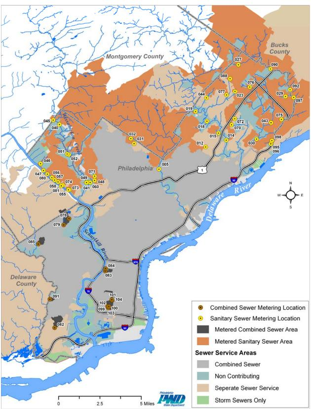
Figure 3-2 PWD Portable Flow Monitoring Program Metering Locations
