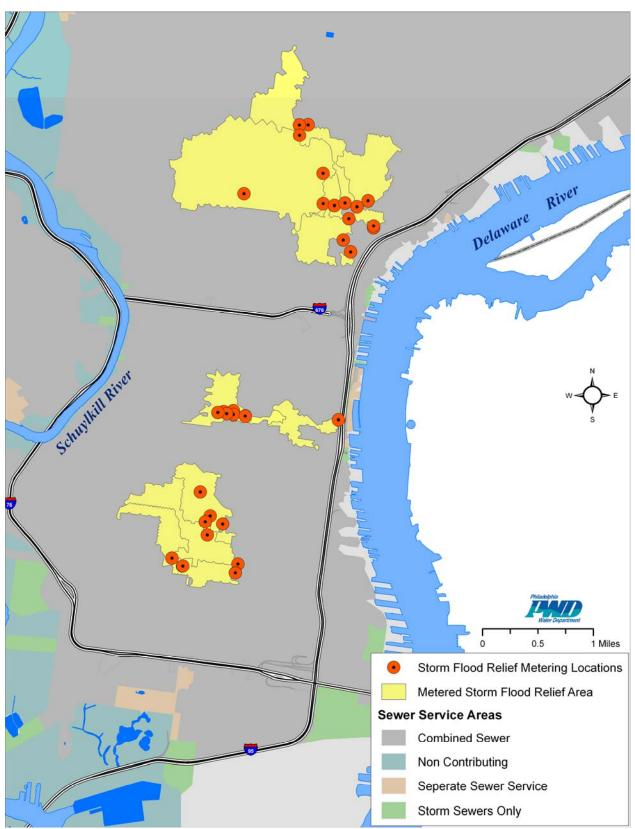
**Figure 3-3 PWD Targeted Storm Flood Relief Monitoring Program Meter Locations** Section 3 • Characterization of Current Conditions
