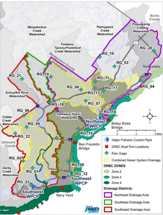
Figure 3-1 PWD Rain Gage Locations and Combined Sewer Drainage Areas
