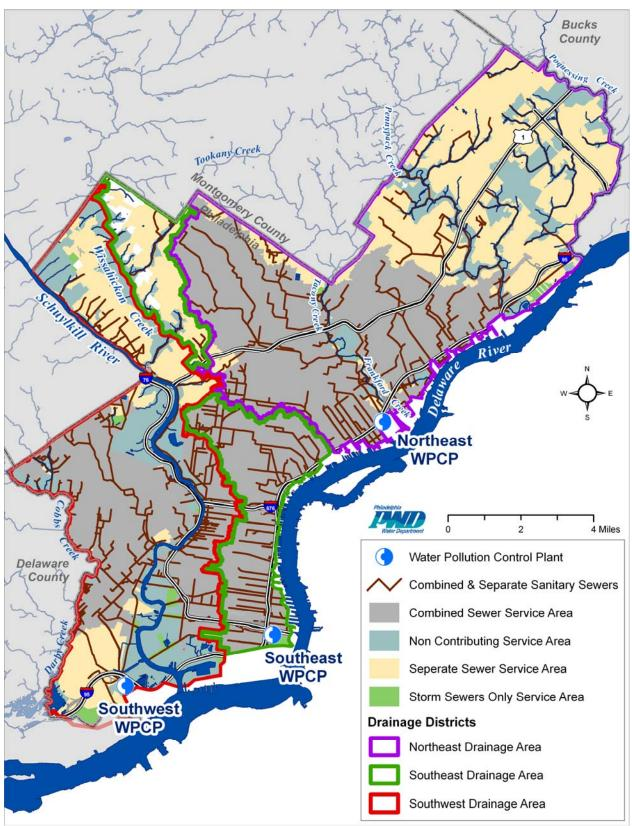
**Figure 3-22 Philadelphia Sewer Area with Drainage Districts Boundaries** Section 3 • Characterization of Current Conditions
