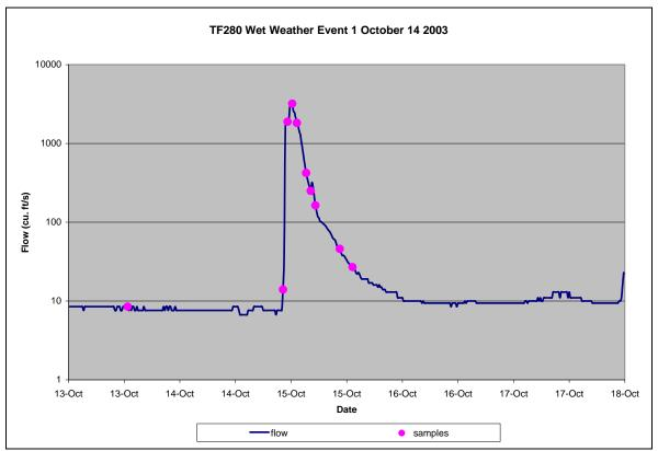
Figure 3-5 Hydrograph Showing Complete Capture of the October 14, 2008 Wet Weather Event from an Automatic Sampler in the Tookany/Tacony-Frankford Creek
