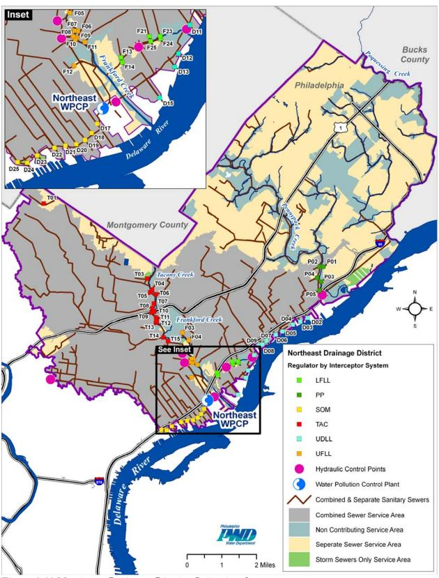
**Figure 3-23 Northeast Drainage District Collection System** Section 3 • Characterization of Current Conditions
