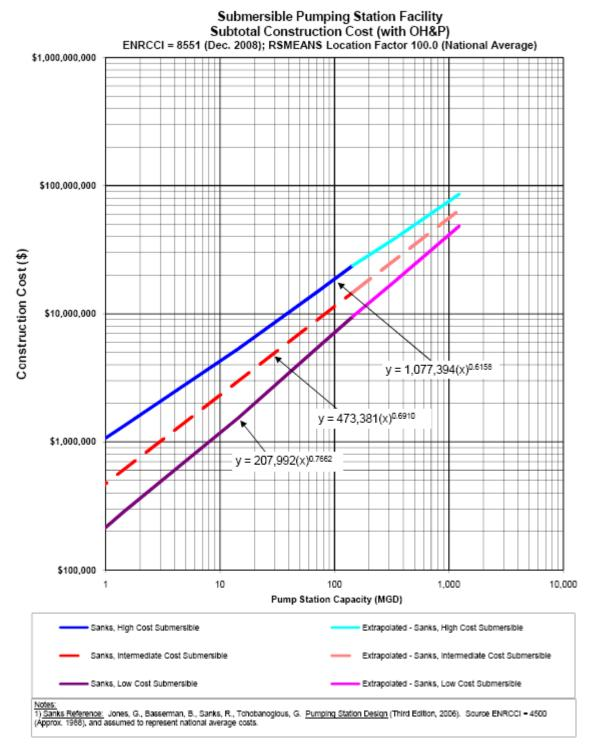
Figure 2.3.6-2 Submersible Pump Station Curves [ENRCCI 8551; RS MEANS 100]
