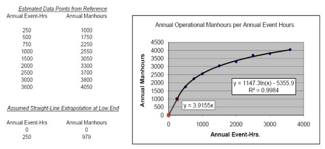
Figure 2.3.13-3 Typical Annual Staff Operation for RTBs [ENRCCI 8551; RS MEANS 100]
