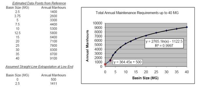
Figure 2.3.13-2 Typical Annual Maintenance Staff for RTBs [ENRCCI 8551; RS MEANS 100]
