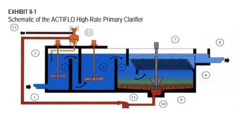
As shown in Exhibit 8-1, the sludge from the ballasted flocculation process is pumped to gravity thickeners to be thickened from 0.3 percent solids to 3-4 percent solids.
