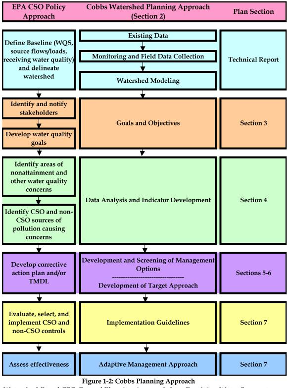
Watershed-Based CSO Control Planning Approach for a Receiving Water Segment – from USEPA Guidance for Long Term Control Plan (1995)
