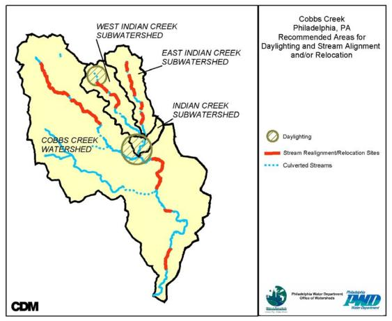
Figure 7-7 Recommended Areas for Stream Realignment and/or Relocation
