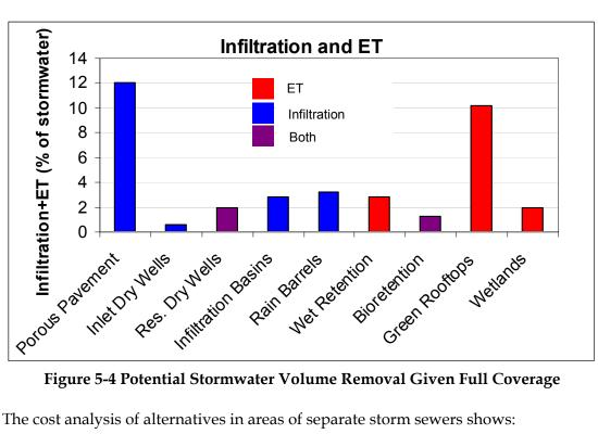
Figure 5-4 Potential Stormwater Volume Removal Given Full Coverage
