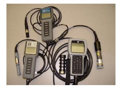
tion. In other cases, the decreases in pH and DO are not as severe, and daily variation returns but with less amplitude and more noise. These problems occur because the sonde's housing has become loaded with debris and sediment, and its mesh screen around the probe guard has become caked with solids. Post-storm cleaning of the mesh screen has shown that once the solids are removed, the sonde returns to capturing data representative of the stream.
