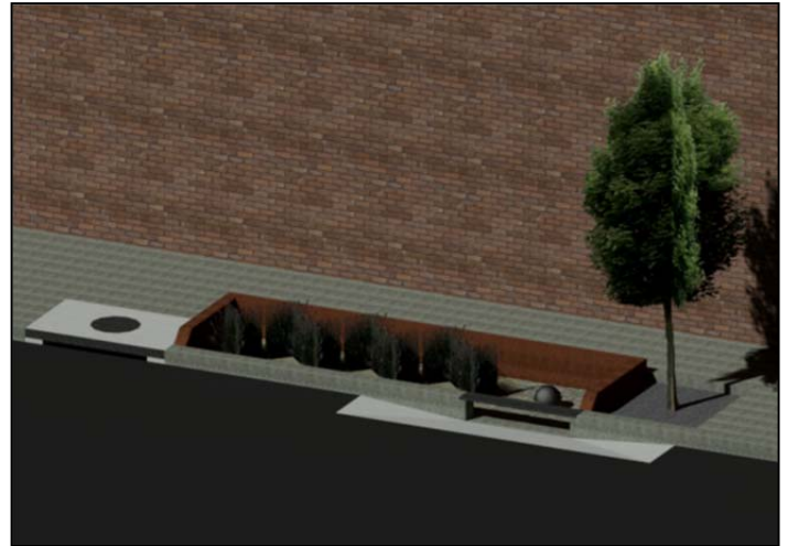
FIGURE 3. The Northern Liberties SFR Projects will have a Green Streets component. Recessed planter beds depicted above filter storm water from the roadway before being discharged to the Delaware River.
