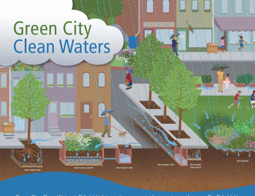
Green City, Clean Waters is Philadelphia's innovative program to clean our rivers and streams. The Philadelphia Water Department uses specially designed green tools to filter and store water through natural processes. These green tools, which often use plants and trees, help stormwater (rain or melting snow) soak into the ground. They are a beautiful and cost effective solution to reduce pollution. This approach will result in greener communities and cleaner rivers that everyone can enjoy.
